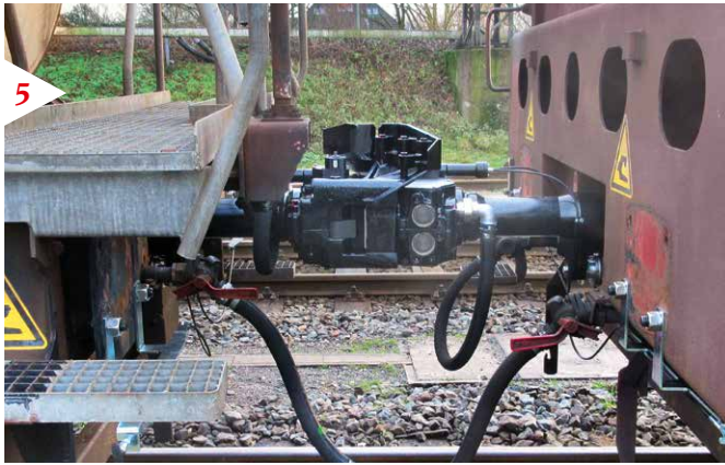
5— Automatic coupler: simplifies shunting processes and optimises train formation activities.
